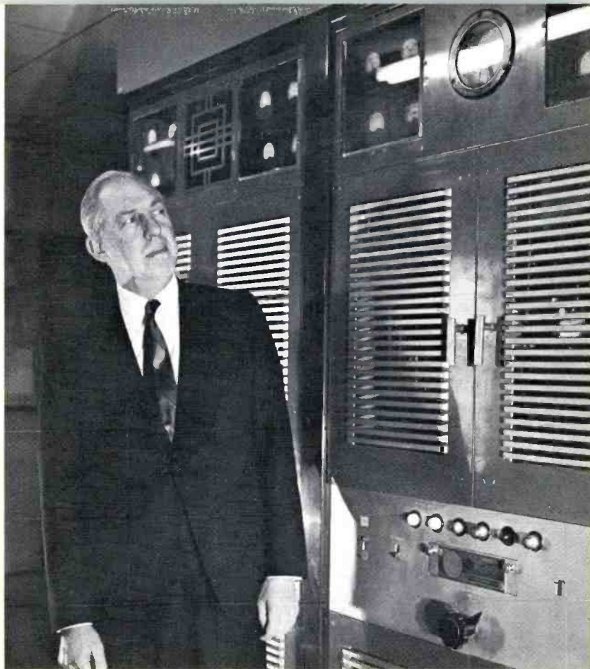
FIG. 15 George S. Johnson, Director, Planning & Research, at RCA Type 10C (used as exciter) which is 5C modified for 10kw output.
