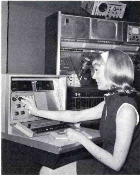
NEW TAPE EDITING SYSTEM was a highlight of the TV tape equipment display. Called a Tape Editing Programmer this new equipment preprograms electronic splicing functions and allows the editor to preview the splice and splice points before actual editing begins. In the photo left the compact unit is mounted in a console to provide remote editing of highband TR-70 in the background.
