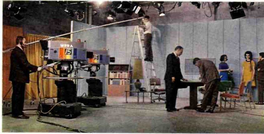
FIG. 8 40' x 60' color studio during preparation for popular live telephone participation show, "Nightline". Two TK-42 color cameras are shown.
