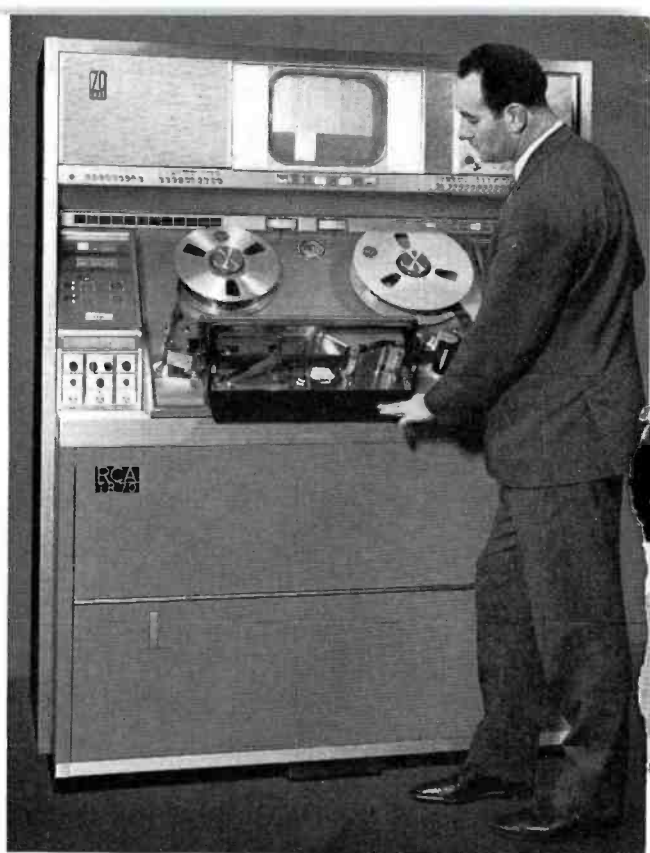
FIG. 4 The Author, P. G. Parker, Chief Engineer, Yorkshire Television Limited, examining one of the two RCA TR-70 television tape recorders.
