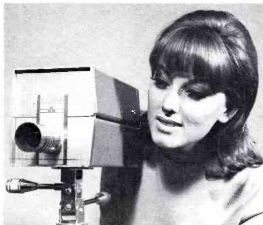
FIG. 3 Solid-state, modular construction permits changing the PK-301 camera to any of thirteen different configurations. It may also be converted to a PK-310 film camera or PK-315 viewfinder camera.
