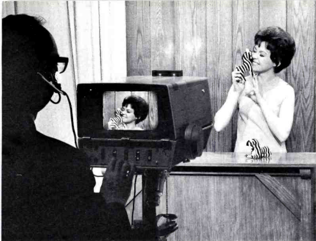
FIG. 1 Lightweight and compact, the PK-330 Studio Camera produces crisp, high-resolution pictures. The camera has built-in pan and tilt functions and a motorized zoom lens.
